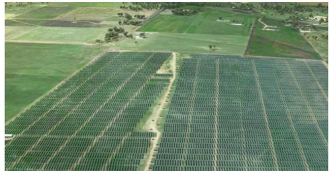
The Moree Solar Farm uses single-axis tracking technology so its 250,000 solar PV panels can tilt to face the sun as the earth rotates. The technology has the potential to produce 30 per cent more energy than a farm using fixed-position panels, and to capture a higher volume of peak priced electricity. The project is also receiving a \$101.7 million Australian Government grant through the Australian Renewable Energy Agency (ARENA).
